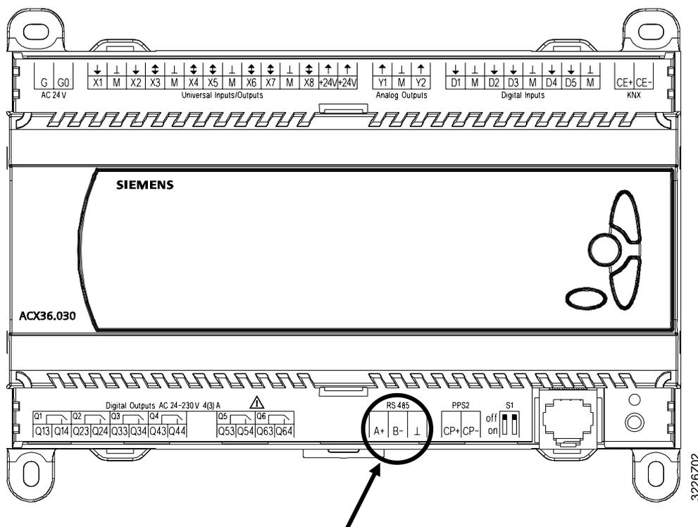
1. Attach communication cable to connector A+ and B-
